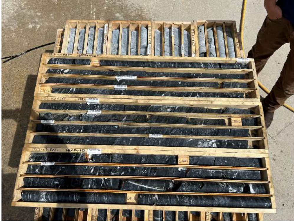
Plate 10-7: Silicified, weakly mineralized Badshot Limestone (679.4-692.2m), drillhole D22-03
