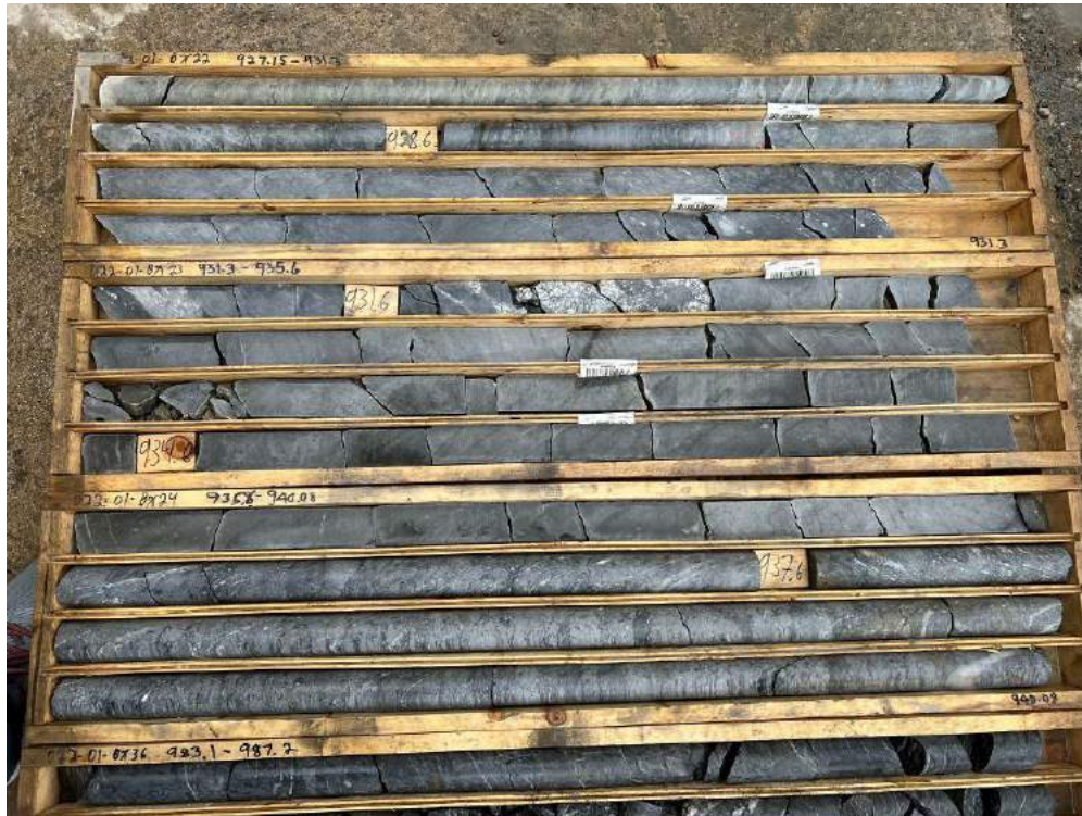
Plate 10-3: Silicified Badshot Limestone (927.15-940.08m), drillhole D22-01
