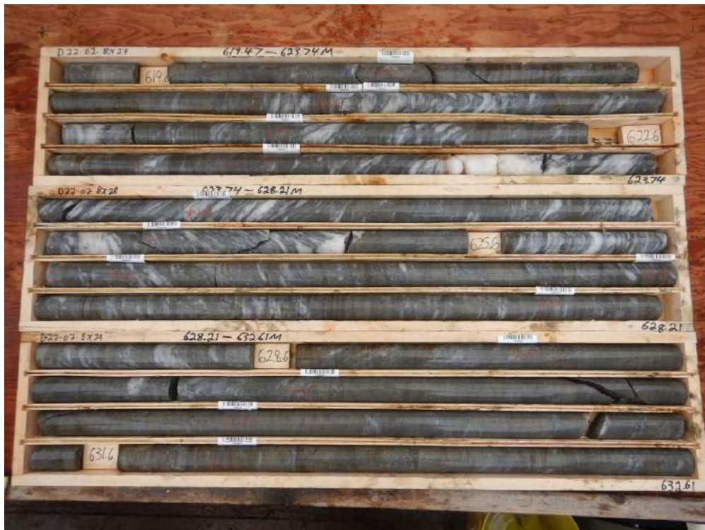
Plate 10-4: Semi-massive to massive sulphide mineralization (619.47-632.61m), drillhole D22-02
