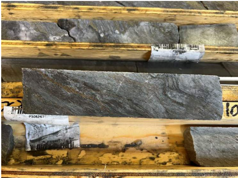
Plate 10-6: Dolomitized Badshot Limestone with wispy sphalerite (647.7m), drillhole D22-02
