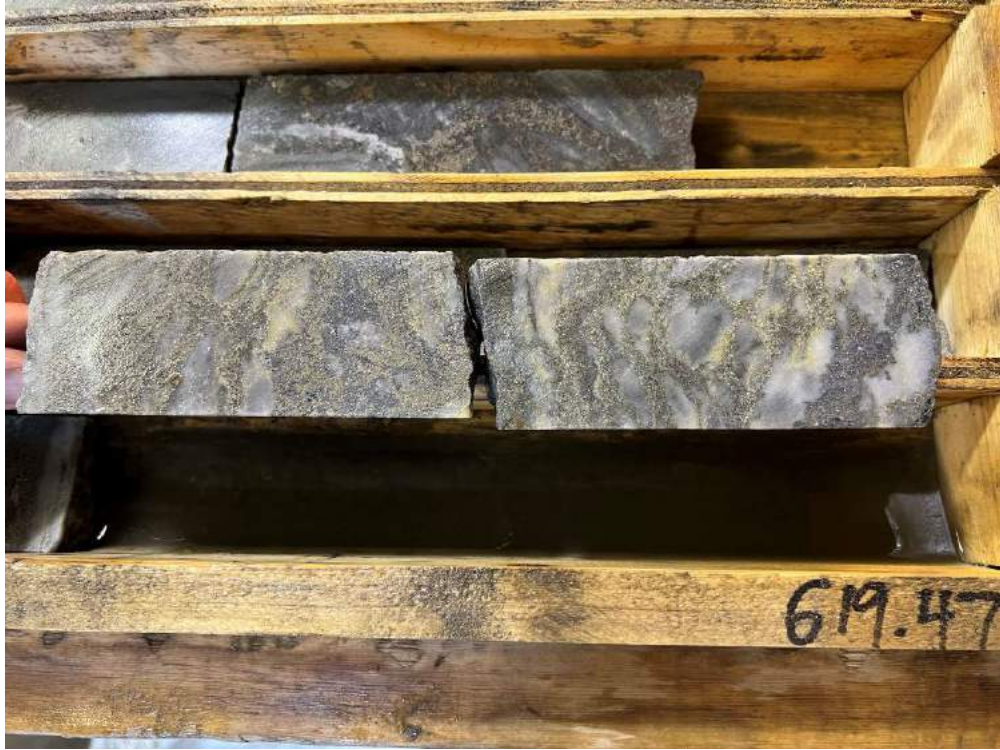
Plate 10-5: Banded pyrite-sphalerite-galena mineralization (619.47m), drillhole D22-02
